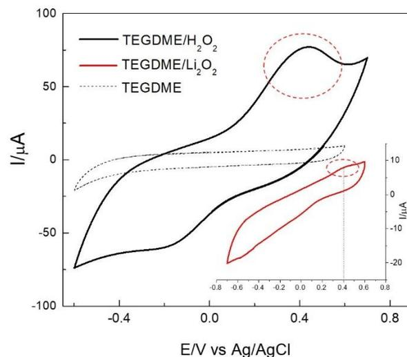
**Figure 1.** Voltammetric profile of platinum electrode in absence (black dotted line) and in presence of 9.8 mM H<sub>2</sub>O<sub>2</sub> (solid black line). Inset corresponds to the voltammetric profile of platinum in presence of 10 mM Li<sub>2</sub>O<sub>2</sub> (solid red line). Red dotted line circle indicates oxidation process. For all systems 0.1M LiClO<sub>4</sub>/TEGDME was used as electrolyte. Scan rate of 100 mV s<sup>-1</sup>.
