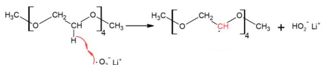
**Figure 3.** Mechanism for the generation of carbon-centered radical species, when the electro-oxidation of  $\text{Li}_2\text{O}_2$  occurs in TEGDME.
