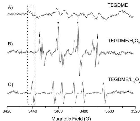
**Figure 2.** ESR spectra of TEGDME in the presence of A) 0.1M LiClO<sub>4</sub>, B) 9.8 mM H<sub>2</sub>O<sub>2</sub> in 0.1M LiClO<sub>4</sub> and C) 10 mM Li<sub>2</sub>O<sub>2</sub> in 0.1M LiClO<sub>4</sub>. The applied potential is 0.4V for 100 scans.
