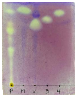
Figure 1: White zones of inhibition; P: Totoralillo plocamium, M: Mertensene, V: Violacene, Compound 3, Compound 4.
